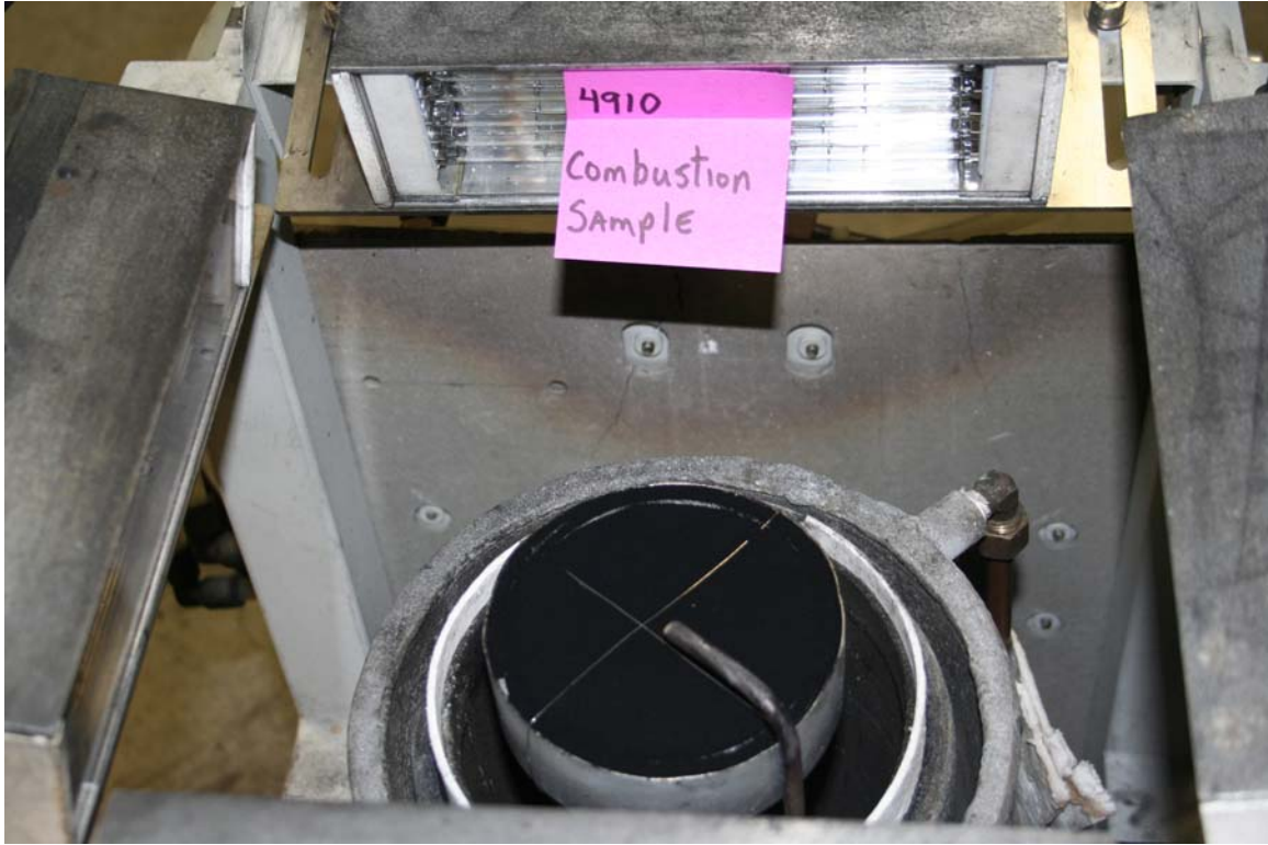
Figure 3: Combustion Test Sample set up on the FPA
