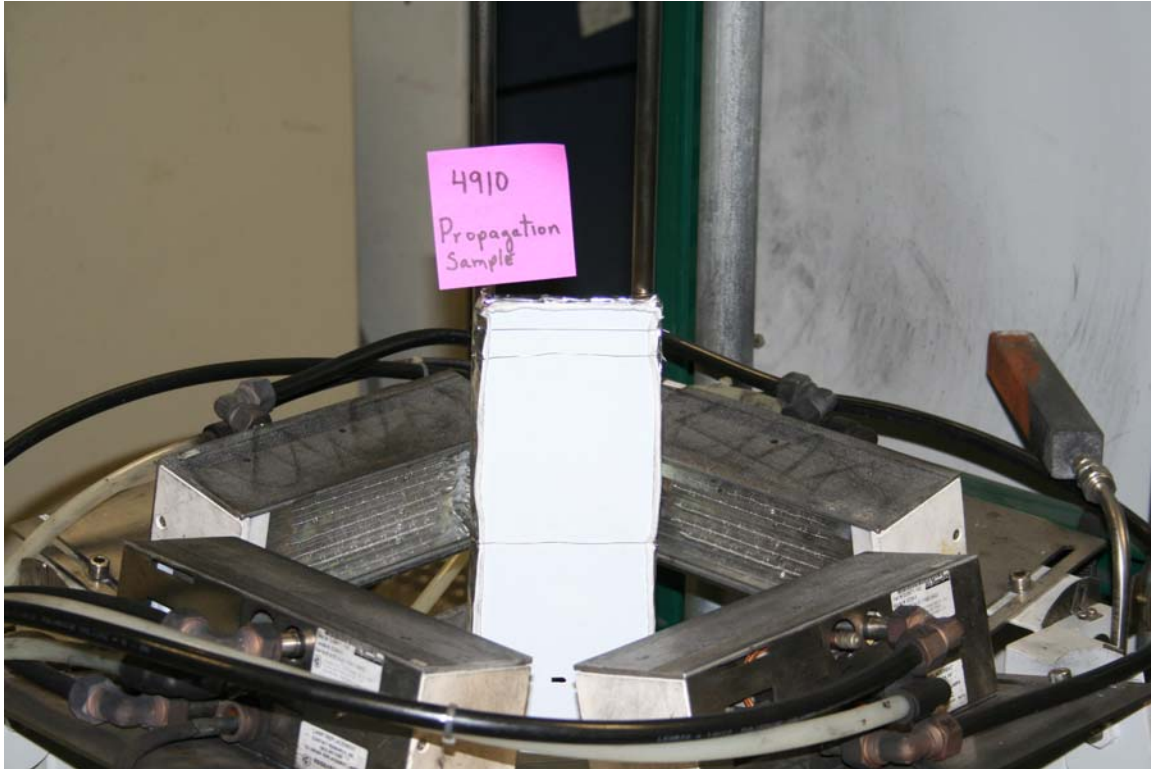
Figure 4: Sample set up on the FPA for Fire Propagation Tests
