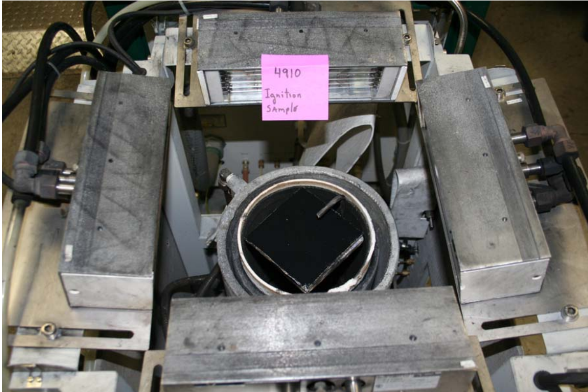
Figure 2: Ignition Test Sample set up on the FPA
